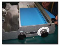
**10.** Slide belt to be skived underneath holding bar and center. The example shown is XH-500-4.
