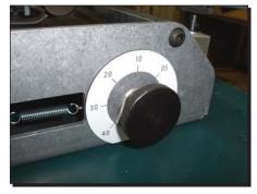
Set thickness knob to the appropriate setting for the belt type being skived. Lock in place.
