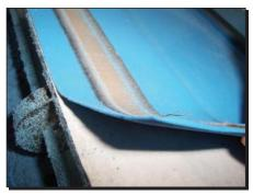
**24.** Skive should taper to thin, feathered edge. Excess material along edge can be trimmed, or sanded down by adjusting nosebar fine-tuner.
