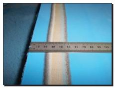
23. Finished skive should have about 10mm width of exposed nylon, centered between sanded rubber areas of equal widths (depending on material).
