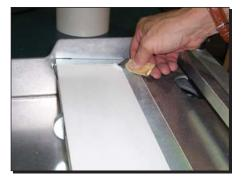
**9.** Peel edge of paper and remove from top side of tape to expose top side adhesive.
