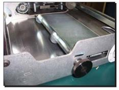
Adjust nosebar fine-tuner knob so sandpaper is as close to steel as possible without touching (sander should slide easily on shaft). Lock in place.
