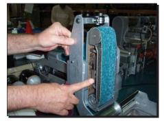
Slide replacement sandpaper onto sander and re-engage locking devices. Lower sander back into place.
