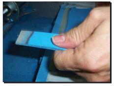
18. If skiving thicker material 12mm from edge, remove belt and any sidebars from tape. If not, skip to Step 21.
