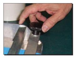
**13.** Tighten both knobs to close holding bar down on belt.
