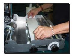
8. Apply piece of double-sided tape across the width of the nosebar. The long edge of the tape should line up with the very edge of the nosebar.
