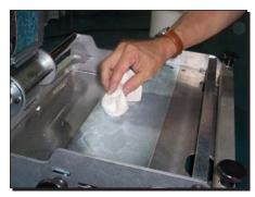
Apply talcum or baby powder to nosebar surface to make double-sided tape easier to remove.
