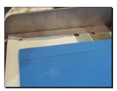
**12.** For wide belts, placing 1" wide sidebars of the same material along both sides of the belt will help to square the skive.
