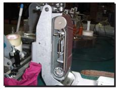
2. If correct sandpaper is already on sander, skip to Step 5. If not, raise sander and disengage locking devices to remove sandpaper.
