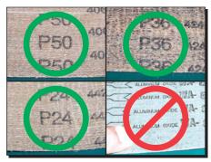
1. Select sandpaper to use based on belt type (see chart below). Grits are clearly marked on back. Use silica carbide paper only, not aluminum oxide.
